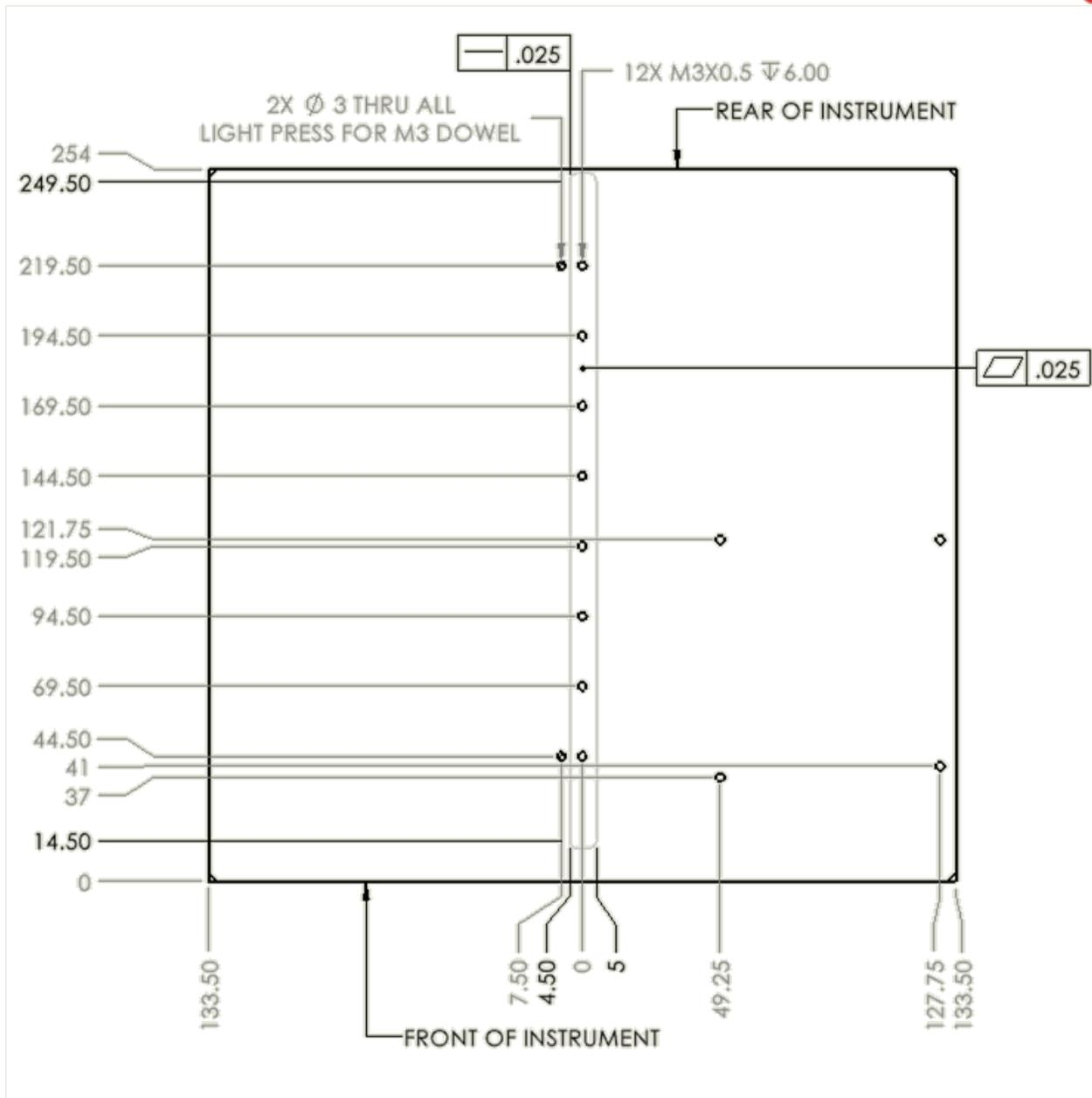
M3x6 socket head fasteners used to fasten the rail should be tightened to 1.0 Nm. Over tightening the fasteners can deform the rail and cause smooth running issues.
