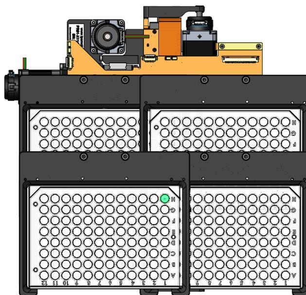
In short, your process will drive the size of your instrument, not the Robot used to carry the microplate around. A minimum footprint of 264mm x 250mm is needed for the Robot to handle the microplate.
