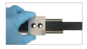
**Step #7** With cap in place you are now ready to insert the socket head fasteners.
