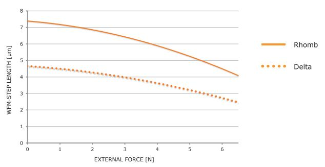
**Figure 1** Motor performance with waveform Rhomb (filled) and waveform Delta (dotted). Wfm-step length is the average distance the drive rod moves when the legs take one wfm-step (i.e. for one waveform cycle). Note: Standard deviation  $\sigma$  of 0.5  $\mu$ m should be taken into account. Typical values are given for 20°C.
